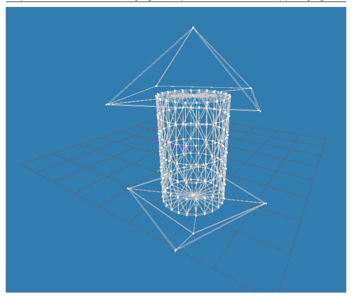
Part of this mesh is a cylinder-like object. As you can see, the surface of it is made of a lot of triangles. The circle-shapes are actually triangles, as well as the jacket surface.
