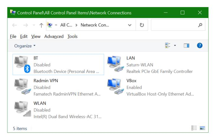
The greyed out elements are the network cards currently deactivated. If you find, that your LAN or W-LAN adapter is actually just deactivated, that would also explain, what is going on. (In the example, the wireless connection is deactivated, the wired connection is active.) In such a case, just activate it (right-click -> Activate, may need administration privileges) and recheck.
