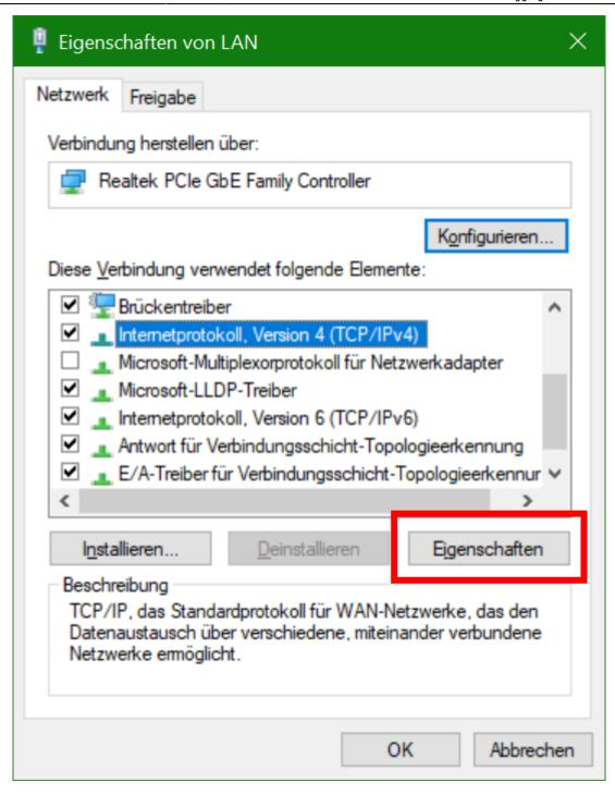
When clicking the *Properties* button after selecting the IPv4 protocol, you can see the current IPv4 settings for that adapter:
