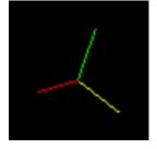
Selected nodes can be moved just as if they were entire models, including their directions. A node is represented by a triad of the three colors red, green and yellow. Their intersection (root) is the location of a node, while the yellow line indicates the direction the node faces. Some tools like Milkshape 3D cannot be used to properly set nodes **and** have them face the correct direction. If you
